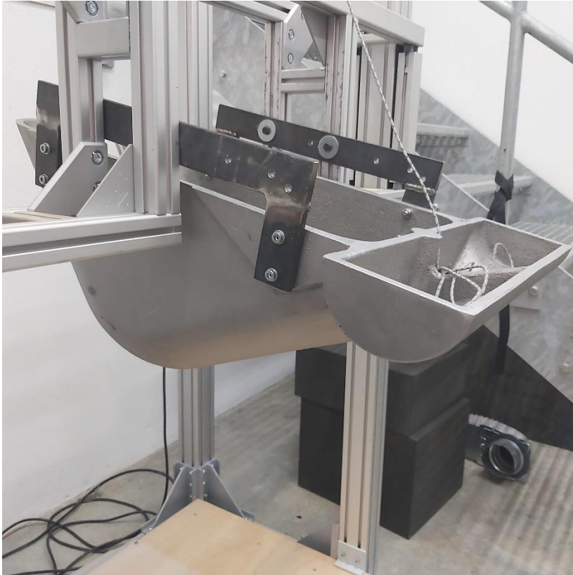
Figure 3: Dummy in 75° leaned back position, DHV-internal test (impact back)
