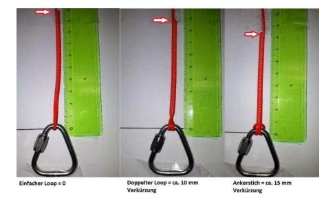
After trim corrections have been made, all lines must be measured again. The tolerances in table 4 apply. In case of trim deviations that cannot be corrected with loops or anchor stitch in such a way that the tolerances in table 4 are met, the manufacturer must be contacted.
